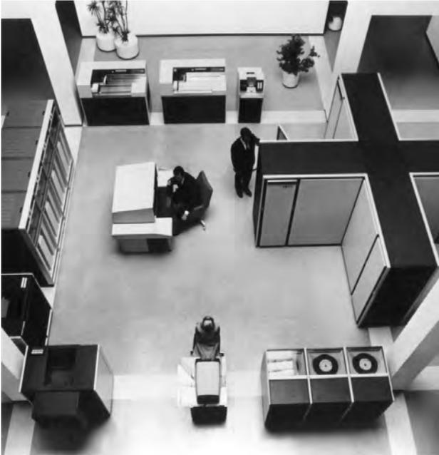
Mainframes were large computer systems that required rooms, designed specifically with raised floors to both conceal the many cables and maintain a constant temperature. Servicing also required specially trained staff, and work was often done in a three-shift operation so as to optimise the use of the system. The picture shows a Cyber installation from the company Control Data Corporation.
