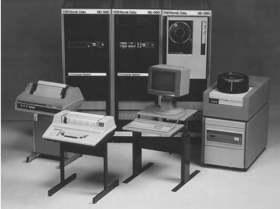
From today's perspective, minicomputers were not exactly mini, but compared to mainframes, they were significantly smaller systems. Moreover, installing a minicomputer was less demanding and whereas many mainframes needed water cooling systems, too, minicomputers were all air-cooled. Shown is a minicomputer system from Norsk Data.
