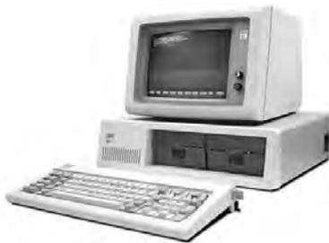
An IBM Personal Computer (PC) with two 5¼" diskette drives and the PC-DOS operating system from Microsoft. The first model, launched in August 1981, is named 5150.
